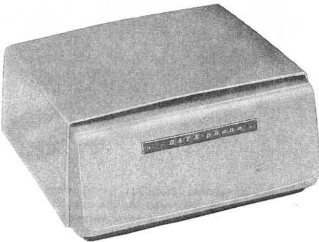
Data Set 103AW type is designed to simultaneously transmit and receive binary serial data on either half or full duplex at rates up to 300 bauds in DATA-PHONE service over the voice message switched network, or at rates up to 150 bauds in TWX service over teletypewriter exchange type facilities.
