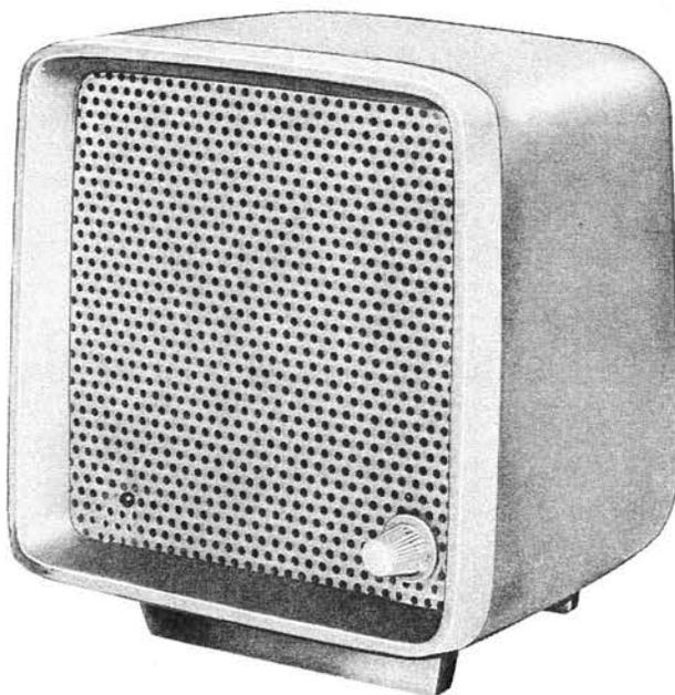
**106A:** Consists of a loud speaker and amplifier assembled on a chassis within a metal housing 5.500 inches wide by 4.625 inches deep by 6.1875 inches high having a green finish. The knob on the right controls an ON-OFF switch and a gain control potentiometer. A 2Y Lamp behind a red jewel indicates the ON condition.
