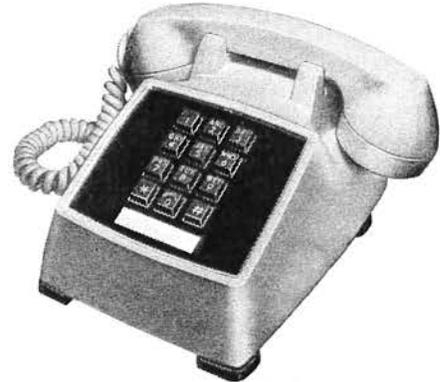
A black common battery desk type TOUCH-TONE telephone set. Equipped with a jack to provide for head telephone set or hand set operation. Equipped with a 253A TOUCH-TONE Dial, a G3AR-3 Hand Set, an N1A Ringer, a 642A Key, a D10P-3 Cord, a 241A Amplifier, a 425G Network, and a 100A Varistor. If Head Telephone Set is required, it must be ordered separately. A snap-on plastic face plate, arranged to accommodate a number card, is mounted on the top side of the housing.
