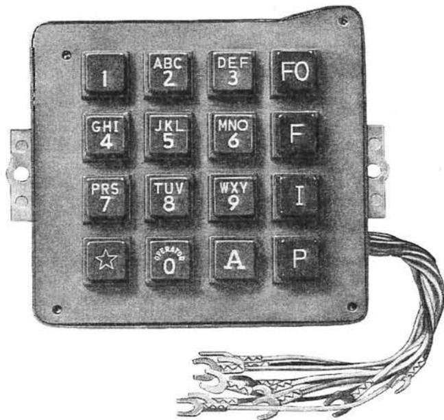
The 66 type dial is a 16 pushbutton multifrequency dialing device. Ten of the pushbuttons, from one to zero, are used for station-to-station calling and the remaining six are used to provide special service signals. Each of the 16 pushbuttons, when operated, generates a double frequency signal distinctive to that button. Overall dimensions are 4.150 inches by 3.397 inches by 1.765 inches. The mounting holes on the mounting bracket are 3.818 inches center to center.
