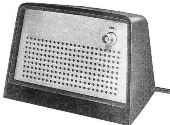
Consists of a KS-16881L5 Loudspeaker and a two-stage transistorized amplifier mounted on a metal base enclosed in a plastic housing. The knob controls an ON-OFF switch and a volume control potentiometer. Overall dimensions are 5.750 inches wide by 4 inches high by 3.750 inches deep.
