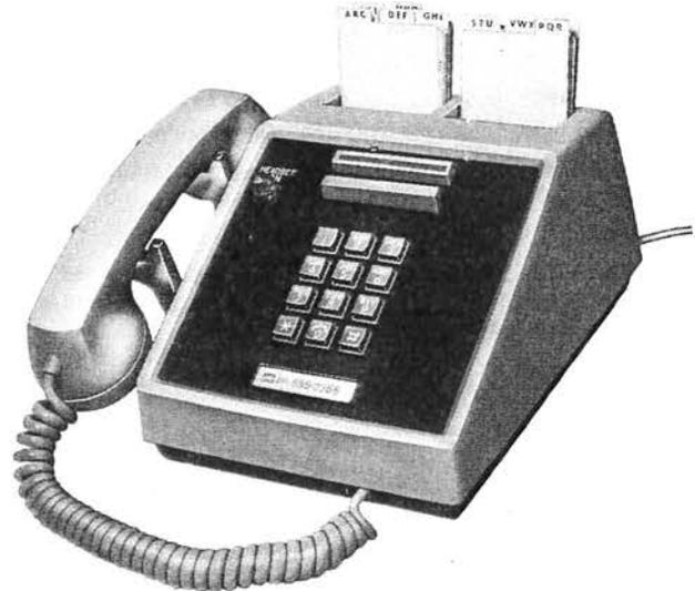
A twelve-button TOUCH-TONE telephone set with overall dimensions of 9.650 inches wide by 9 inches deep by 4.381 inches high. Equipped with a D6AF Type Mounting Cord.
