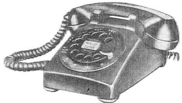
Common battery desk type that provides improved performance transmission, dialing, and ringing functions. These gains can be used either for extension of range of operations from central office or increased use of fine gauge cable conductors. Volume of the ringer may be varied in four steps. By removing the housing and making a minor adjustment, the ringer can be silenced.
