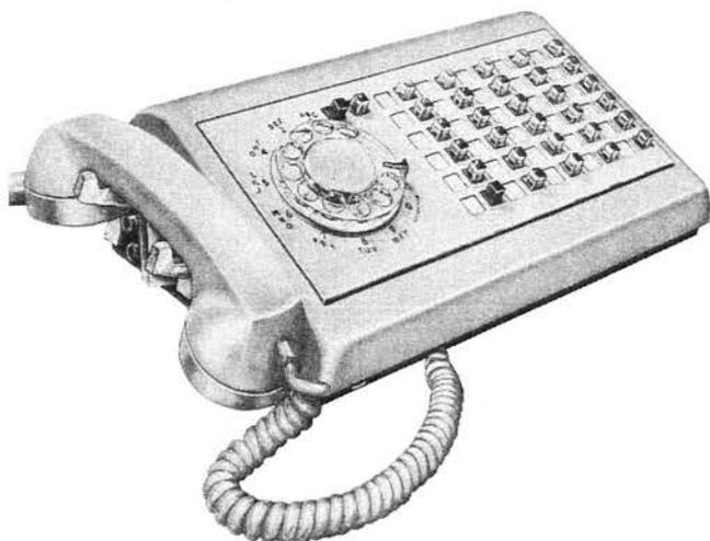
A general purpose five-position key telephone set with overall dimensions of 15.125 inches wide by 8.125 inches deep by 4.226 inches high.
