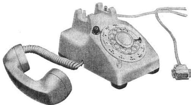
A common desk type telephone set which provides an interlock feature between the telephone line and a data set. The set is light gray and has overall dimensions of 8.297 inches wide by 9 inches deep by 4.906 inches high. The set has an exclusion type data key (left plunger) for voice-to-data transfer.
