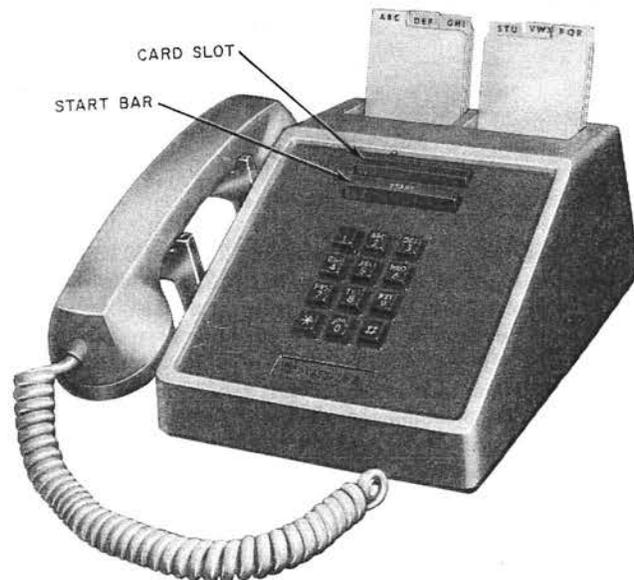
2660AW1: A twelve-button TOUCH-TONE type telephone set with overall dimensions of 9.650 inches wide by 9 inches deep by 4.381 inches high. Equipped with a D3BN Type Mounting Cord.
