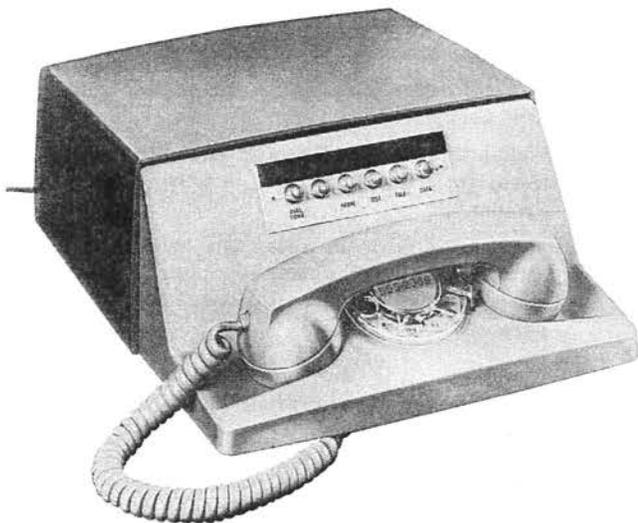
**402CW1:** This is an integrated unit which combines a telephone set and a transmitter component of a medium speed, binary, parallel data transmission system. Provides unattended answering, alternate voice transmission, and data transmission of any number of binary data levels up to 8 at any speed up to 75 characters per second. Also provides timing signals and a nonsimultaneous answer-back feature at a maximum operating speed of 20 two-bit characters per second.
