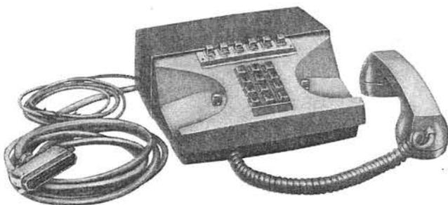
804GW1: Consists of a two-tone gray plastic housing containing an 11C Apparatus Unit, a 589T Key, three 52A Lamps, a D4BJ-61 Cord, an M14F Cord, and printed wiring boards containing component apparatus.
