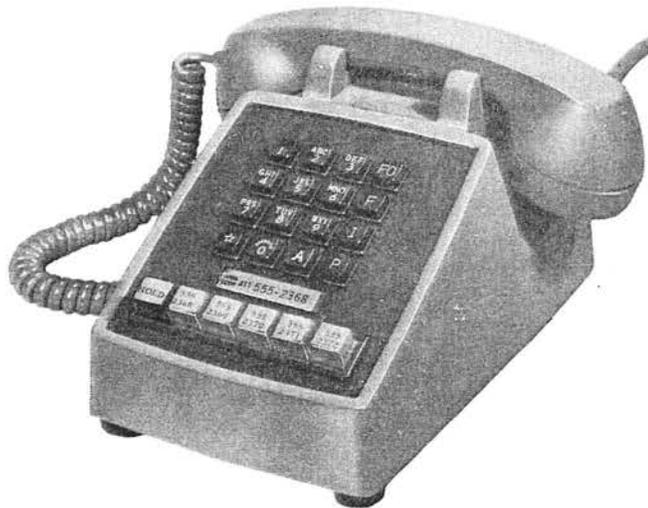
A common battery, desk type, telephone set arranged for two- or four-wire service. The sets are factory wired for four-wire service. Overall dimensions are 8.312 inches wide by 9 inches deep by 4.906 inches high.
