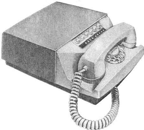
The 202EW type Data Set is an FM transmitting data terminal integrated with a rotary dial telephone set in a two-tone gray plastic housing. Provides normal point-to-point transmission of voice or of serial digital information at data transmission rates up to 1200 bauds on the switched network or up to 1800 bauds on some private line facilities. Designated for voltage signal interface.
