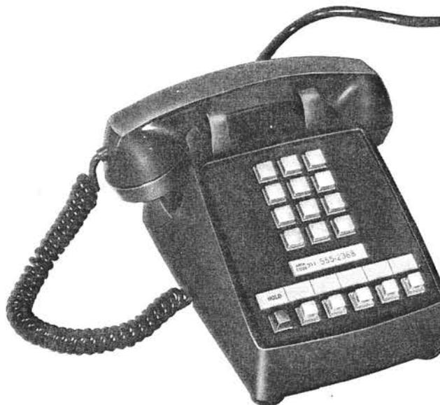
A desk type, common battery, 12-button TOUCH-TONE dial telephone set equipped with a line switch which provides six transfer contacts and is arranged for two-wire service. The set is convertible to four-wire service at installation. Overall dimensions are approximately 8.297 inches wide by 4.906 inches high by 9.000 inches deep.
