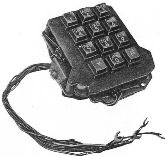
Each is a 12-button TOUCH-TONE dial. Ten buttons are used in a number-letter dialing and two are used to give special service connection and are identified by an asterisk and a pound symbol. Overall dimensions are approximately 3.425 inches by 3.531 inches by 1.790 inches.
