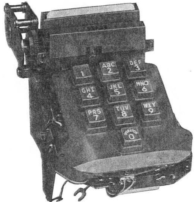
A combination TOUCH-TONE dial and a card reading mechanism for multifrequency dialing manually or from a coded card. One P-24E238 Card Set is furnished.
