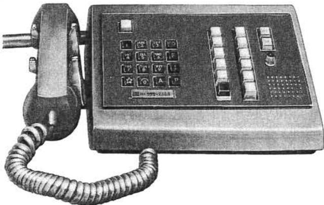
A desk type telephone set in a plastic housing with a sloping top surface having overall dimensions of 12.5 inches wide by 8.250 inches deep by 4.226 inches high. Has a clear, antiglare plastic face plate (P-29E340) and a coordinated colored mat which are assembled in a stainless steel bezel which snaps in place and can be readily removed from the housing for maintenance.
