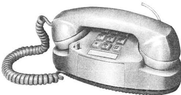
and surge protector, and other component apparatus. The lamp is used for dial illumination and may also be operated as a night light.
