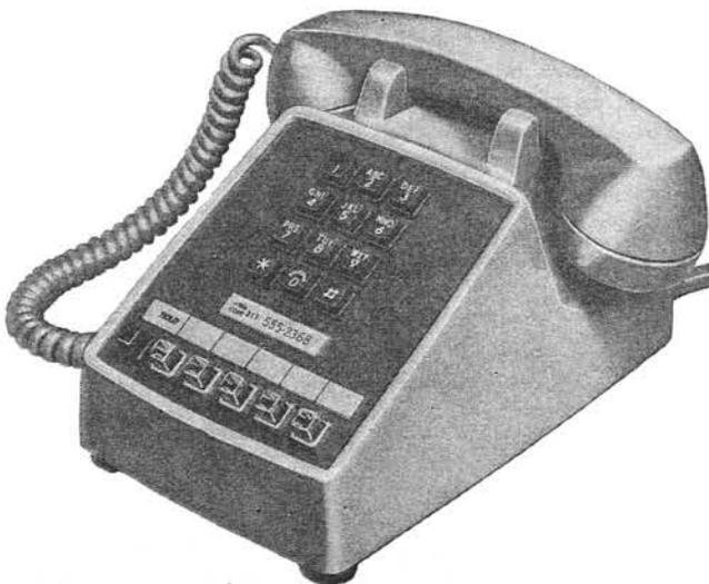
A desk type, common battery, TOUCH-TONE dial, six-button key telephone set arranged for two-wire service and equipped with a line switch which provides six transfer contacts. The set is convertible to four-wire service at installation. Overall dimensions are approximately 5.625 inches wide by 9.556 inches deep by 5.234 inches high.
